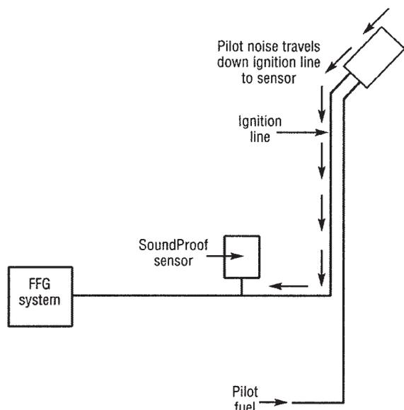
**Figure 4.** SoundProof® Acoustic System.
