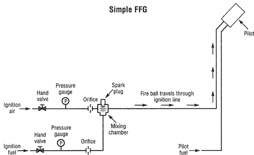
Figure 2. A simple flame front generator (FFG).
