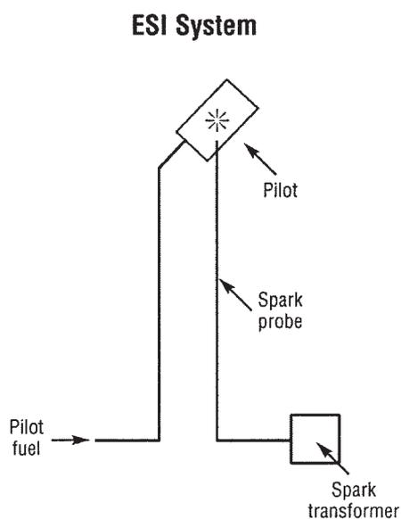
Figure 3. An Electronic Spark Ignition (ESI) pilot.
