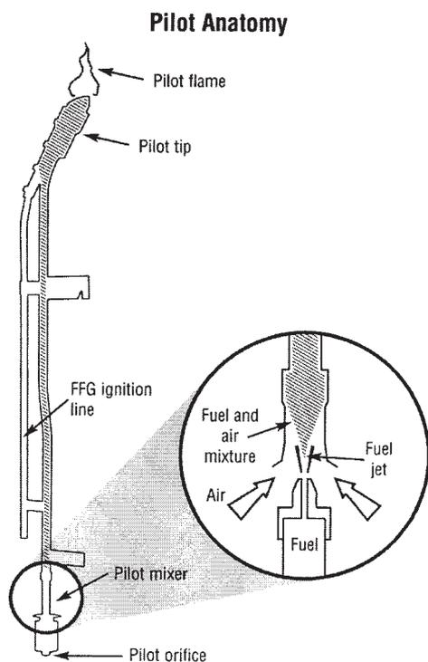
**Figure 1.** A typical pilot assembly.
