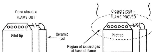
**Figure 5.** Flame ionization system.
